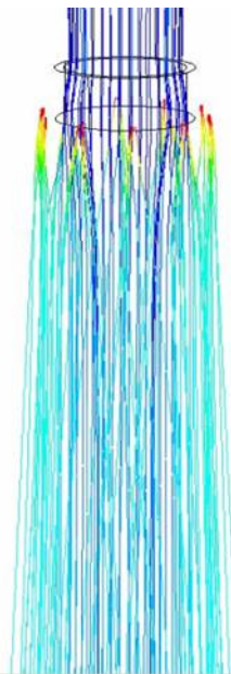
Figure 8. Pathlines of fuel jets and combustion air.
