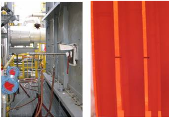
Figure 7. CO sampling to determine flame length.
